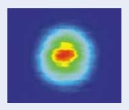
Typical PHAROS near field beam profile at 200 kHz
